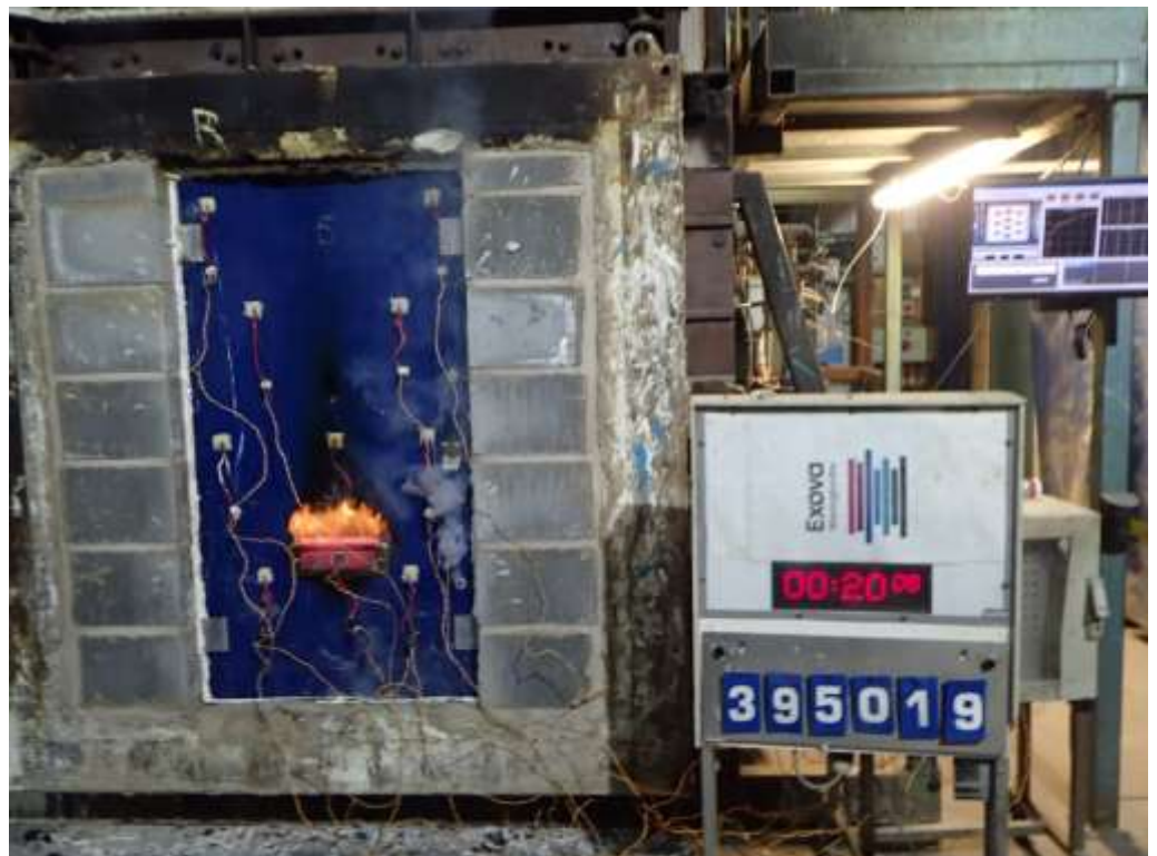
The unexposed face of the doorset after a test duration of 20 minutes
