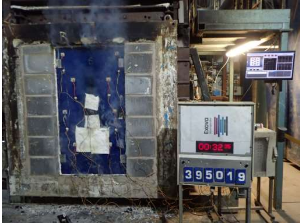
The door viewer on the unexposed face of the doorset is blanked off after a test duration of 32 minutes
