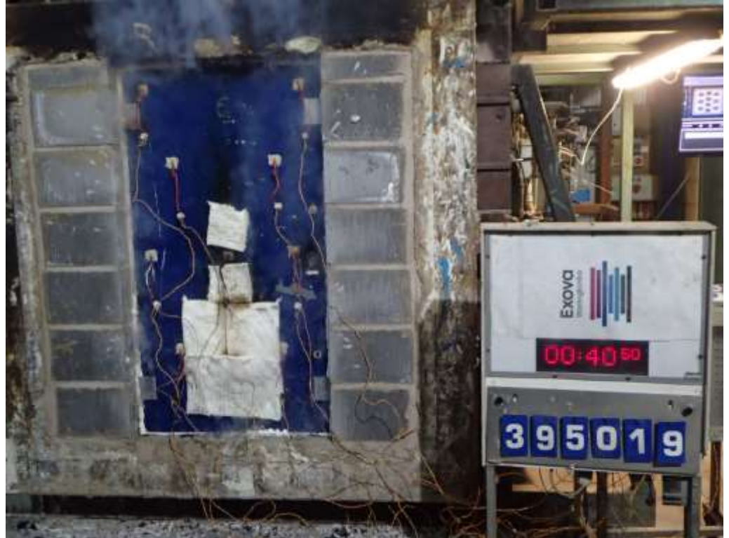
The unexposed face of the doorset after a test duration of 40 minutes
