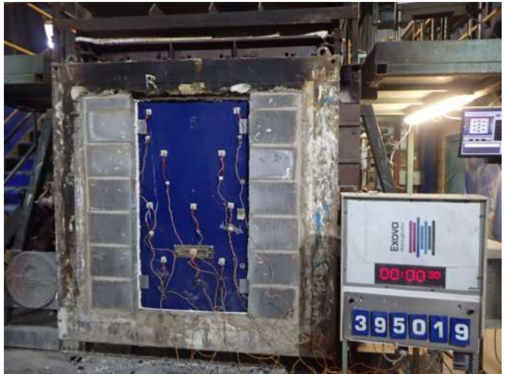
The unexposed face of the doorset prior to testing
