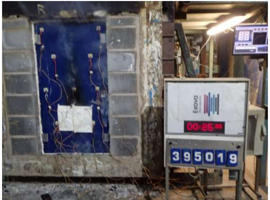
The unexposed face of the doorset after a test duration of 25 minutes
