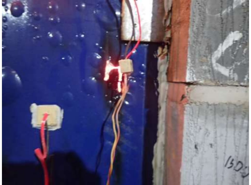
Holes beginning to form on the unexposed face of the doorset after a test duration of 43 minutes
