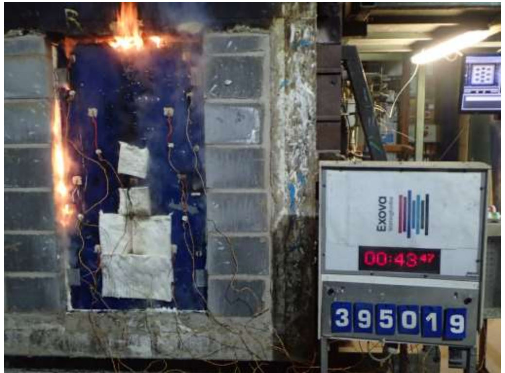
The unexposed face of the doorset after a test duration of 43 minutes
