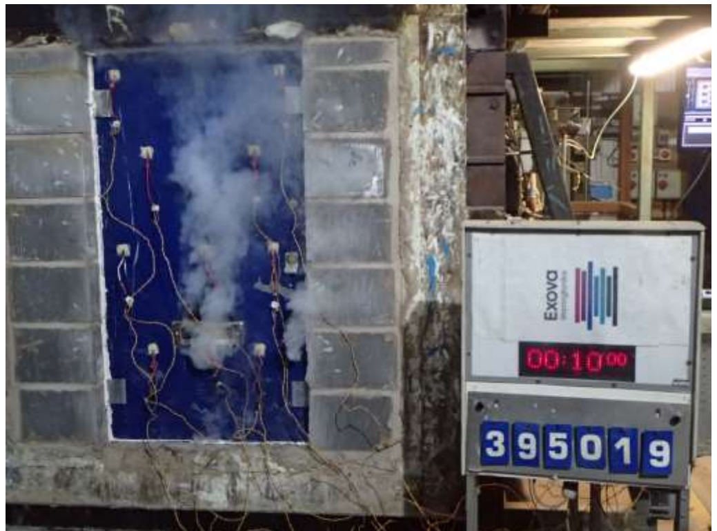
The unexposed face of the doorset after a test duration of 10 minutes
