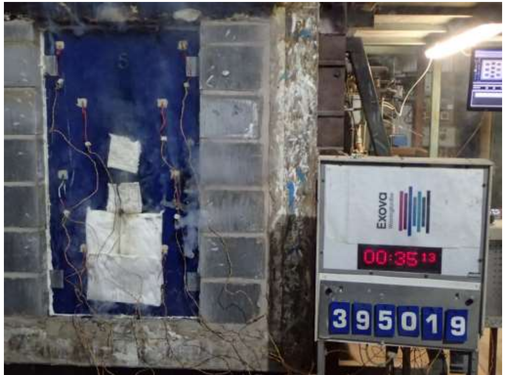
The unexposed face of the doorset after a test duration of 35 minutes
