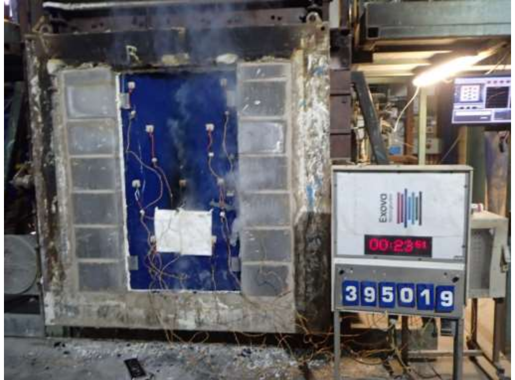
The letter plate on the unexposed face of the doorset is blanked off after a test duration of 23 minutes
