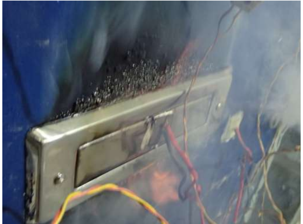
Flaming observed from around the letter plate on the unexposed face of the doorset after a test duration of 14 minutes
