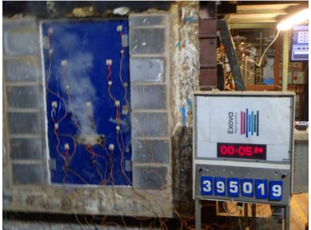
The unexposed face of the doorset after a test duration of 5 minutes
