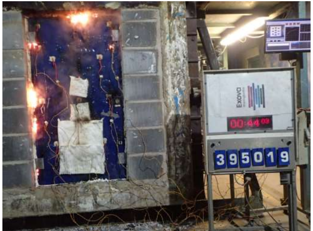
The unexposed face of the doorset after a test duration of 44 minutes
